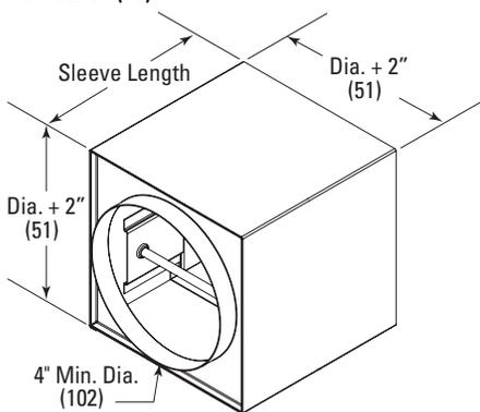
Square to Round transitions external on both ends of the damper sleeve. Product is ordered on duct Diameter; damper will be fabricated 2" (51) larger in width and height. Collar extends 1.25" (32) beyond the sleeve length.
