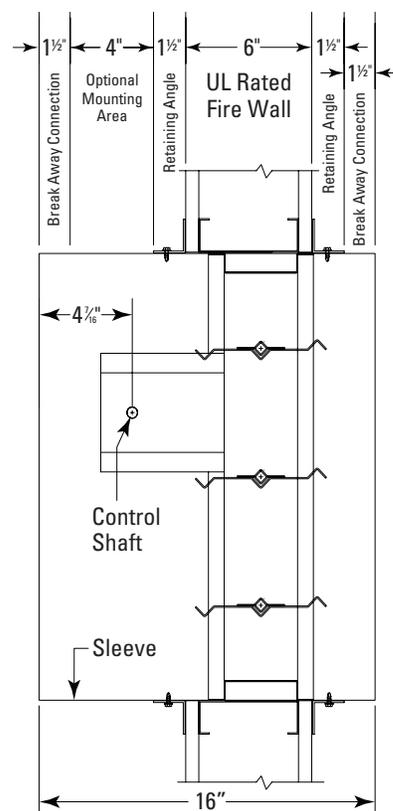
Sleeve Detail for Factory Mounted Sleeve
