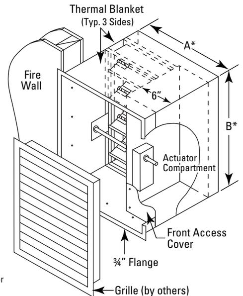
\*Width [A dimension] and Height [B Dimension] are approximately 1/4" undercut. Sleeved dampers are furnished approximately same size as given duct dimension plus 0.25" (6) for insulation.
